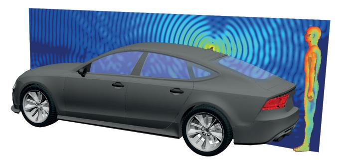
3D EMPIRE model of vehicle with bystander showing electric field and specfic absorbtion rate (SAR) in body model
